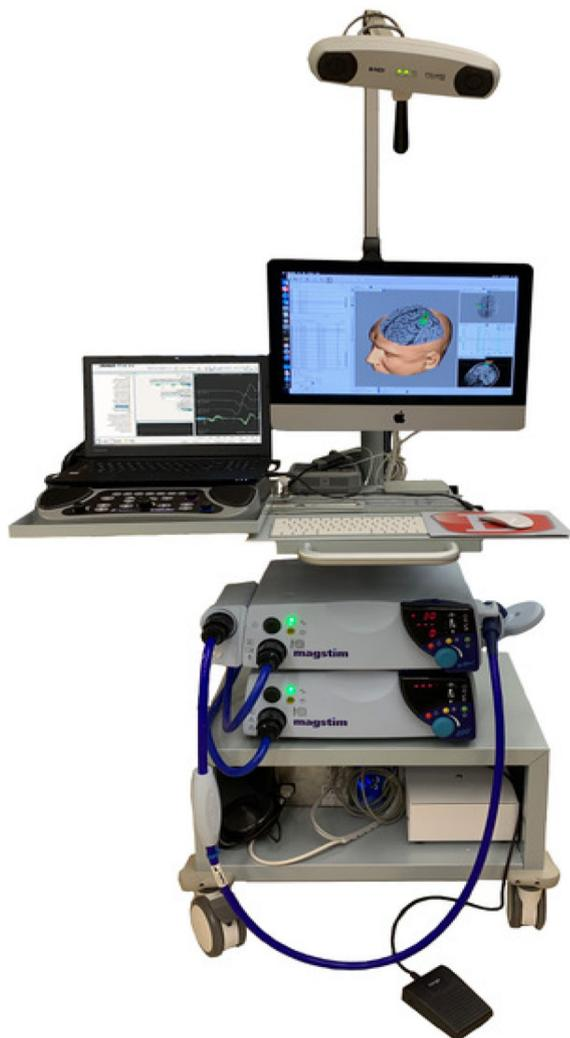
**Fig. 1.** A transportable cart equipped with a TMS unit, a 70-mm figure-of-eight remote coil, and a neuronavigation system. A reconstructed brain image with real-time feedback of coil location was used to guide the stimulation in the primary motor cortex. This cart can be wheeled into a ward and this setup allows TMS assessments to occur acutely at the bedside.
