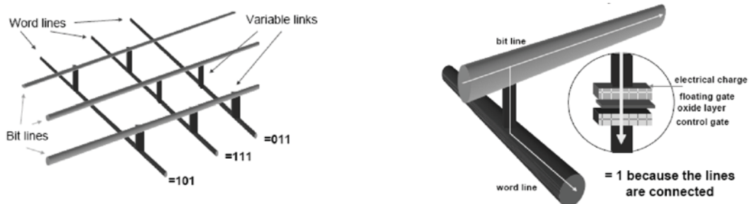
Fig. 2 Basic design of memory chip (left) and flash memory links (right) (O’Kelly, 2007)
