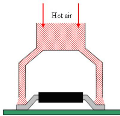
*Extracting TSOP Using Hot Air Method Figure 3*
