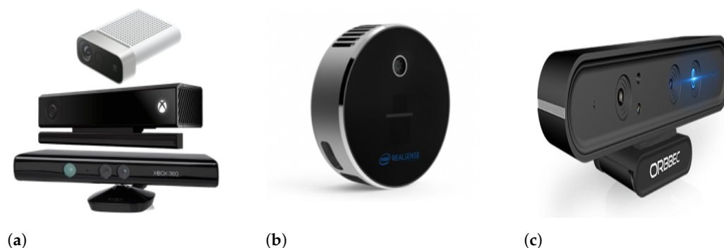
Figure 3. Various RGB-D sensors: (a) Microsoft Kinect [33–35], (b) Intel RealSense L515 [36], and (c) Orbbec Astra Pro [37].
