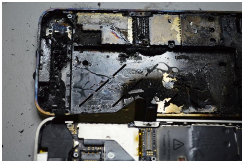
Figure 8: Heat damaged iPhone 4S (top) normal iPhone 4S bottom
