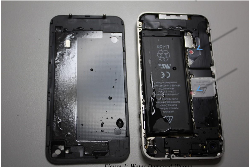
Figure 1: Water Damaged iPhone 4S
