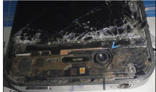
Figure 3: Friction damaged iPhone 4
