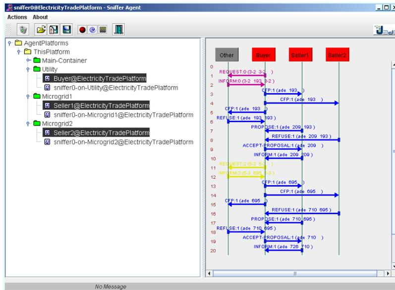
Figure 5. Smart electricity trade process using multi-agent technology
