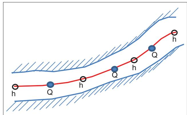
Figure 2: Schematic nodding of h-points and Q-points for a river section in MIKE11 model<sup>[7]</sup>
