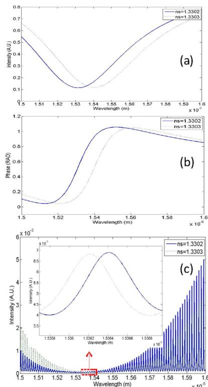
Fig. 2. (Color online) (a) SPR reflection  $r_{\text{SPR}}$ , (b) phase shift  $\phi$ , and (c) transmitted intensity  $I$  versus wavelength for the SPR-based optical FP sensor, for  $n_s = 1.3302$  and  $1.3303$ .
