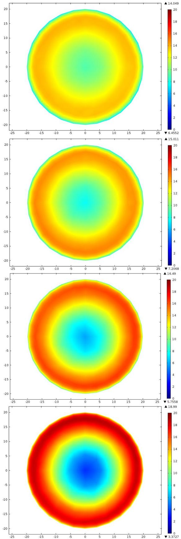
**Figure 5.** The effects of changing straight section length on the uniformity of velocity magnitude at the exit plane for Re = 30,543 and axial-to-tangential flow = 0:100. (From the top: L = 423mm, L = 323mm, L = 223mm, L = 123mm)
