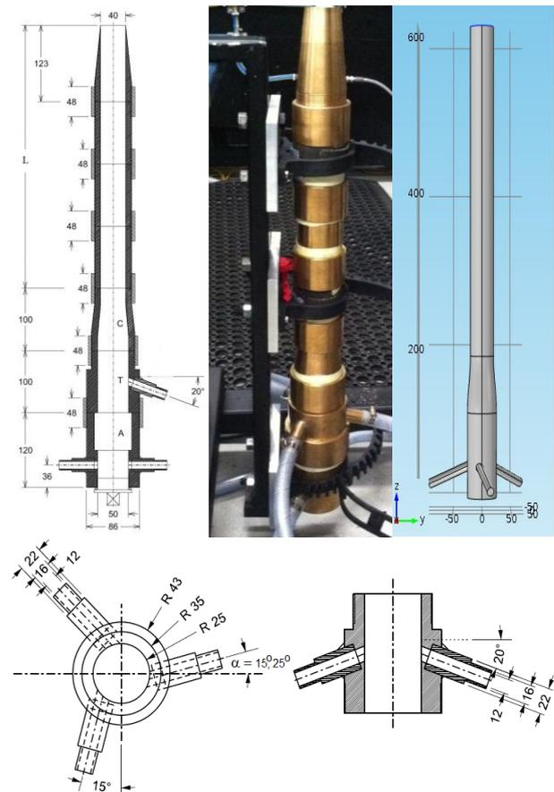
**Figure 1.** Nozzle dimensions (top - left) and the length of the straight section which was varied ( $L=123\text{mm} - 423\text{mm}$ ). Also shown is the final manufactured nozzle (top centre), the fluid domain modeled using CFD (top right) and the angle of tangential ports which was varied (bottom left,  $\alpha=15^\circ$  or  $25^\circ$ ). The port inclination off the horizontal (bottom right) was always  $20^\circ$ . Images not to scale.
