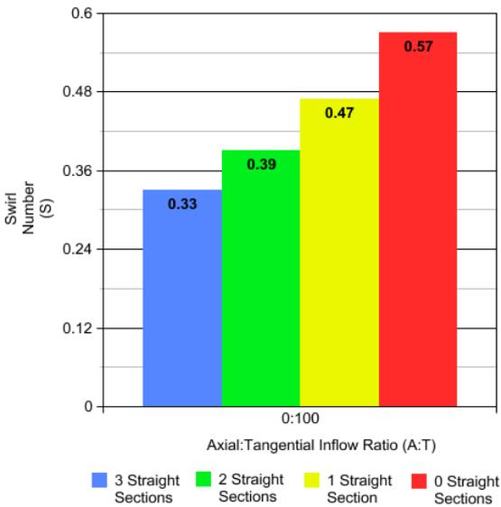
**Figure 4.** Predicted swirl numbers at different lengths upstream of the exit plane for Re=30,543 (L=123 for 0 straight sections, L=223 for 1 straight section, L=323 for 2 straight sections and L = 423mm for 3 straight sections). Fig 1 shows dimension L.
