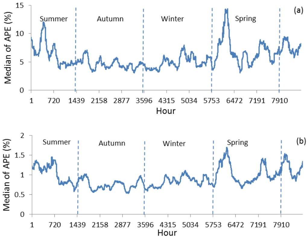
**Figure 6:** Prediction errors using 168 hour input data of wind speed (only) for the years 2007-2009: (a) FF-NN; (b) RBF-NN. The first day in the figure corresponds to 1<sup>st</sup> January.
