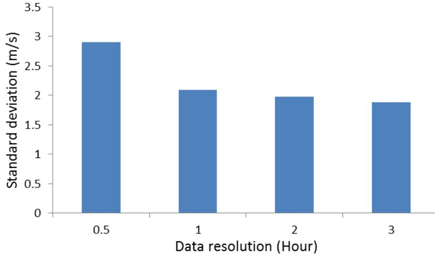
**Figure 9:** Standard deviations of the wind speed training data with different resolutions.
