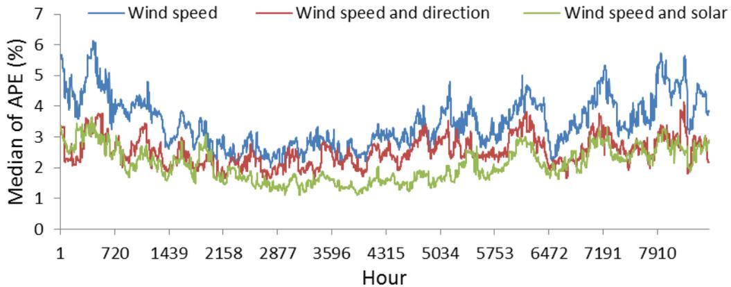
**Figure 8:** The effect of prediction parameters on the accuracy of wind speed predicted via FF-NN over the years 2007-2009 (LTP=10 hours). Different combinations of (historical) meteorological data are used as inputs when attempting to predict wind speed. Hourly resolved data is used in training the Neural Network.
