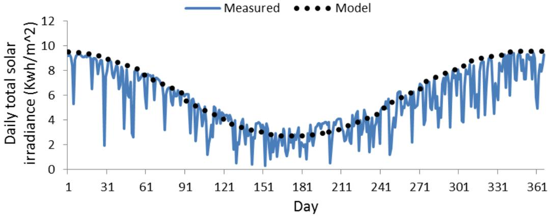
**Figure 2:** A comparison of daily (cumulative) total solar irradiance derived using the ASHRAE model compared to measured (meteorological) daily totals data. (latitude:  $-31.75^{\circ}$ , longitude:  $115.8^{\circ}$ , 2004).
