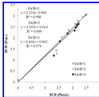
**Figure 7. Comparison of experimental and numerical BCR**
