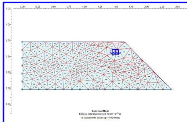
**Figure 3. Deformed mesh for the optimum condition**
