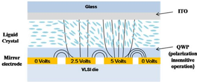
Fig. 1. Opto-VLSI processor layout, Opto-VLSI cell structure and pixel architecture.
