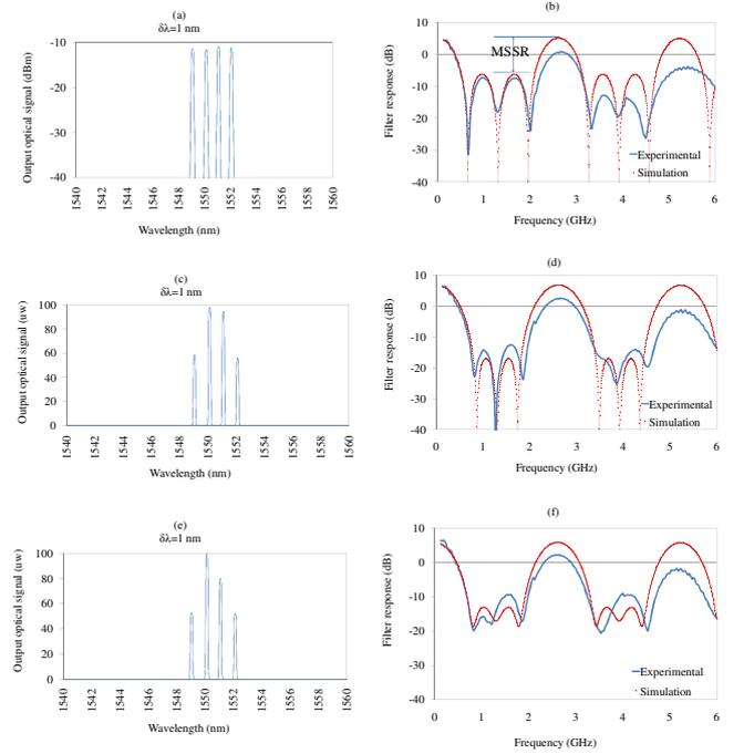
Fig. 4. (a), (c) and (e) Weight profiles of the four WDM RF-modulated channels and (b), (d) and (f) corresponding RF filter responses. Weight profile in (a) is  $[1, 1, 1, 1]$ , in (c) is  $[0.6, 1.0, 1.0, 0.6]$ , and in (e)  $[0.5, 1.0, 0.8, 0.5]$ . WDM channel spacing is 1nm centre-to-centre.
