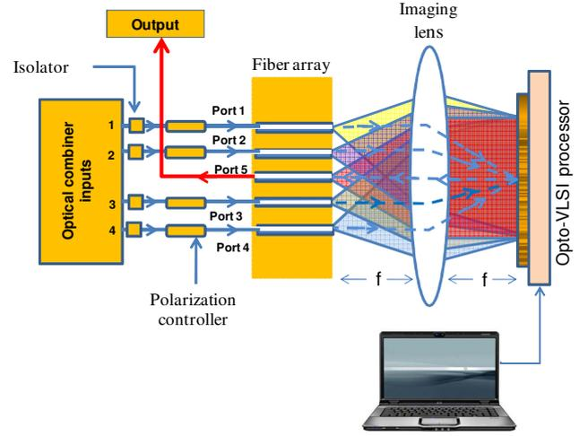
Fig. 2. Opto-VLSI based adaptive optical signals combiner structure.
