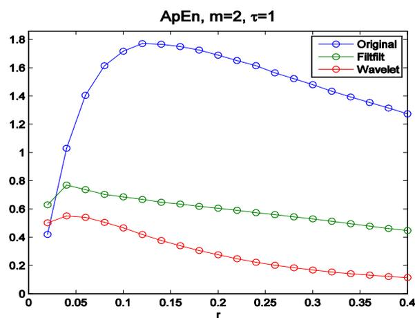
Figure 5. ApEn value of original and filtered signal.
