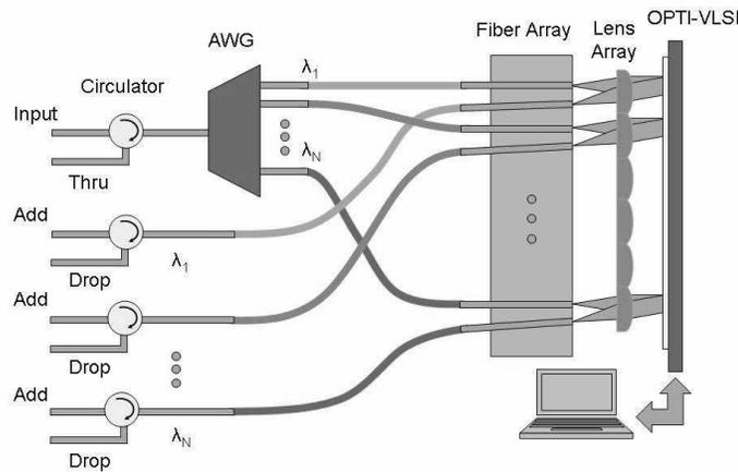
Fig. 5. A ROADM structure with multiple add/drop ports.
