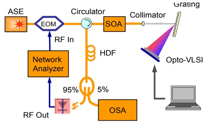
Fig. 2. Tunable time delay structure and Experimental setup
