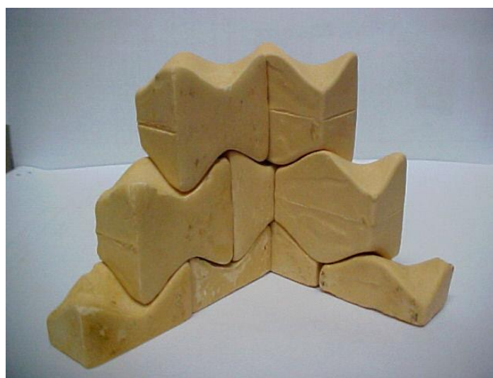
Figure 1. Topological interlocking shapes and structure “Reprinted/adapted with permission from Ref. [15]. Copyright 2015, Dyskin et al.”
