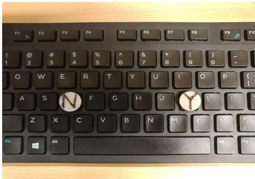
Figure 2. Tactile pads representing “YES” and “NO” responses, covering the “D and “K” keyboard keys.
