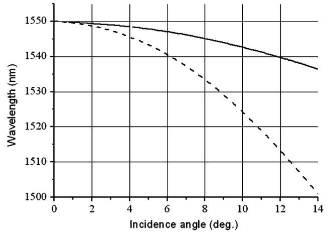
Fig. 8. MPC operational wavelength as a function of incidence angle for the structure  $(NM)^{12}(MN)^1(NM)^1(MN)^{12}$  sandwiched between (i) air and glass ( $\varepsilon_a = 1, \varepsilon_b = 2.310$ ) (solid line), or (ii) two identical media index-matched to the mean refractive index of the structure ( $\varepsilon_a = \varepsilon_b = 3.168$ ) (dashed line).
