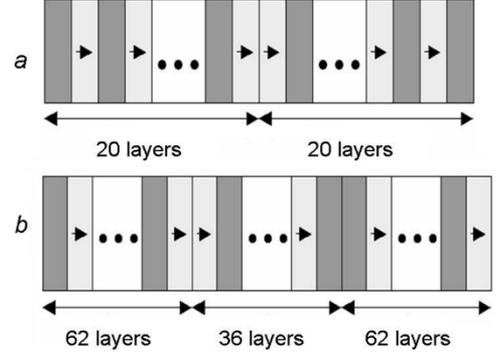
Fig. 2. Structures of  $(NM)^{10}(MN)^{10}$  (a) (with one defect) and of  $(NM)^{31}(MN)^{18}(NM)^{31}$  (b) (with two defects).
