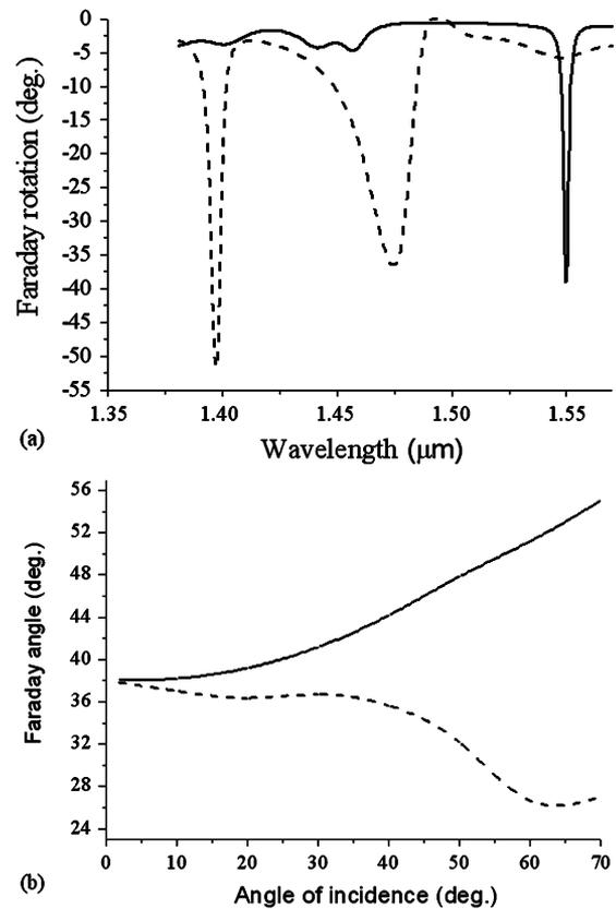
Fig. 6. Faraday rotation for the MPC of formula  $(NM)^{20}(MN)^{20}$ . (a) Faraday rotation spectra for the s-polarization at normal (solid line) and oblique (incidence angle is  $63^\circ$ ) (dashed line) incidence. (b) Faraday rotation for s- (solid line) and p-polarizations (dashed line) at the peaks versus incidence angle.
