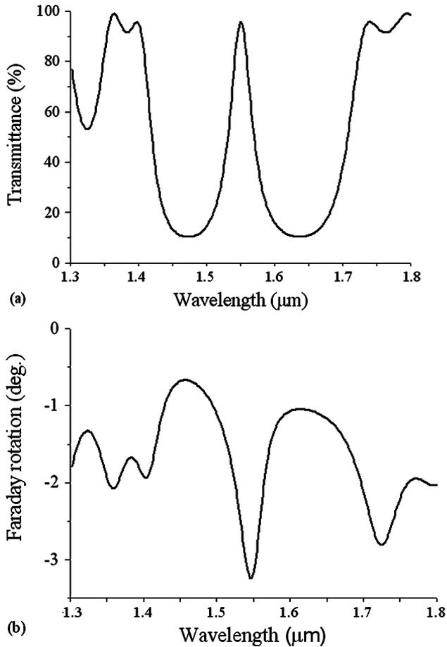
Fig. 3. Transmittance (a) and Faraday rotation angle (b) spectra for the MPC of formula  $(\text{NM})^{10}(\text{MN})^{10}$  in the case of normal incidence.
