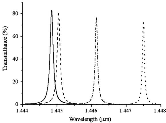
Fig. 5. Transmittance peak position of the p-polarization incident on the MPC of formula  $(NM)^{31}(MN)^{18}(NM)^{31}$  at the  $50^\circ$  angle for four different magnetic layers gyrations:  $g = 0$  (solid line),  $g = 0.01$  (dashed line),  $g = 0.03$  (dash-dotted line), and  $g = 0.05$  (dotted line).
