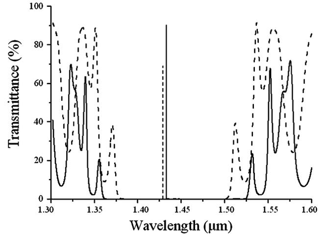
Fig. 4. Transmittance spectra for the MPC of formula  $(\text{NM})^{31}(\text{MN})^{18}(\text{NM})^{31}$  at the  $50^\circ$  incidence angle for two basic incident polarizations: s- (solid line) and p- (dashed line).
