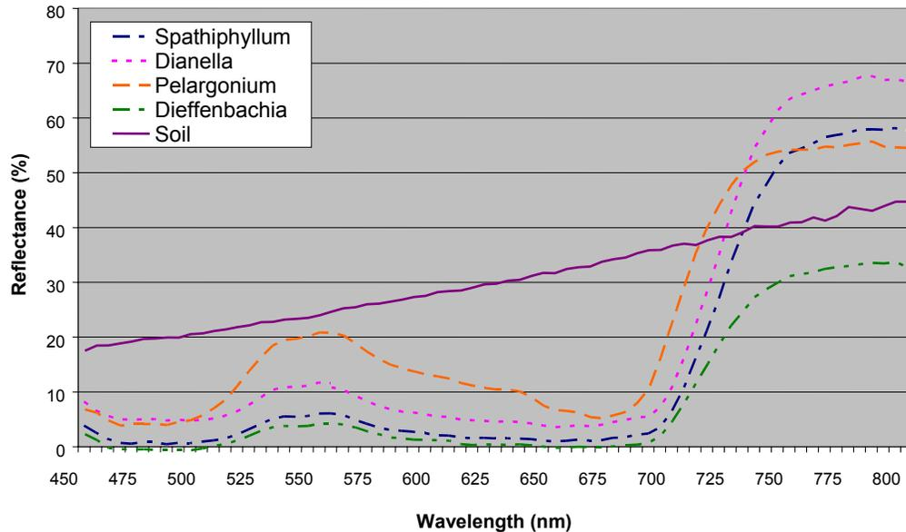
Fig. 8. Spectral response of plants and soil used for experimentation.
