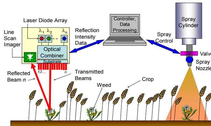
Fig. 2. The sensor will emit light at varying wavelengths along one optical path, striking the same spot on the leaf, stem or soil. Processing of the digitally recorded reflected light signal for each wavelength will determine plant or soil identification and hence a strike signal is sent to the spray valve accordingly.
