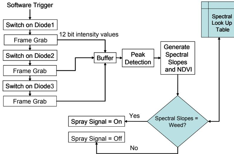
Fig. 7. Flow chart for a single acquisition cycle. This cycle must be completed before the farming vehicle has traveled 4mm – the spot diameter of the projected beam. This is to ensure each of the three frames grabbed is from the same spatial points on the plant or soil.
