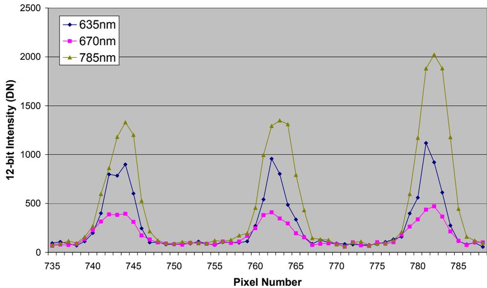
Fig. 6. Gaussian intensity profile of three spots striking a green leaf recorded by a line scan imager.
