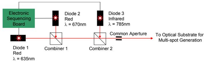
Fig. 3. Laser beam combination.
