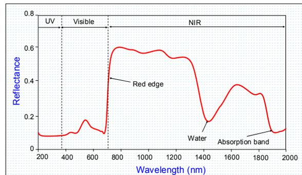
Fig. 1. Typical reflectance spectrum of a green leaf. Variations in the reflectance of the 'red edge' between 650nm and 800nm can be used to discriminate between different plants.
