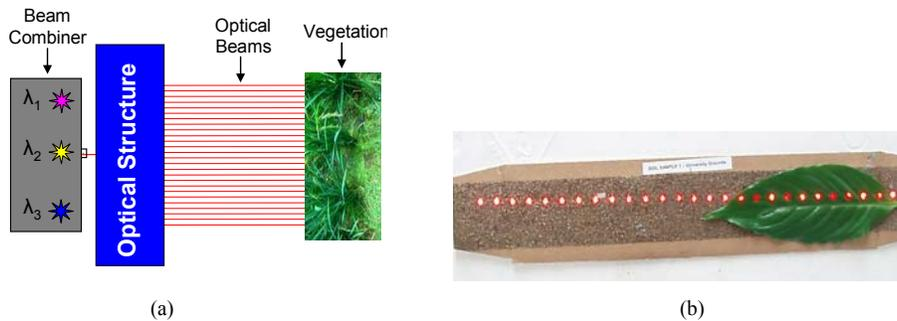
Fig. 4. (a) Multiple beam projection. (b) Resulting spot array projected onto an experimental screen holding a leaf over background soil.
