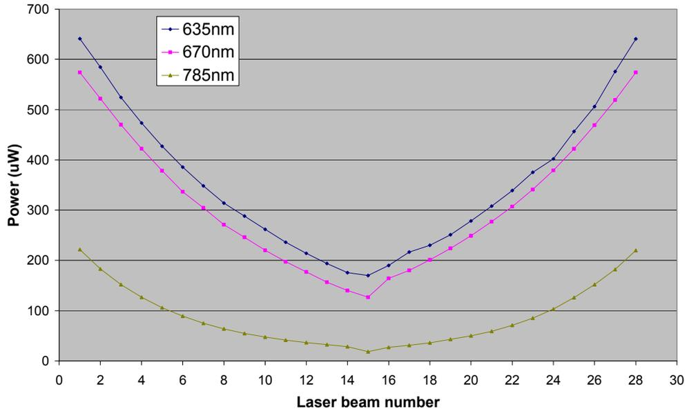
Fig. 5. Measured optical power for each spot projected from two adjacent cavities at each wavelength.
