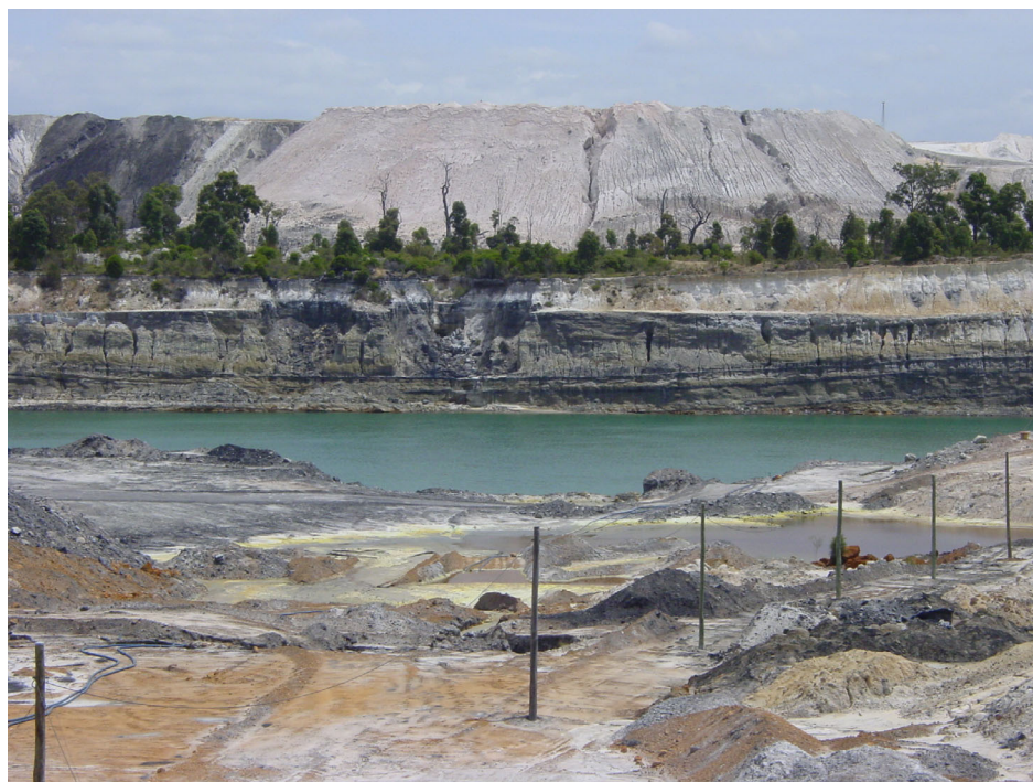
FIGURE 2 The open-cut mining process creates mountains of overburden (background). Re-filling the pit requires extensive dewatering and earthmoving. Photo by M. Lund, 2004, Western Australia.
