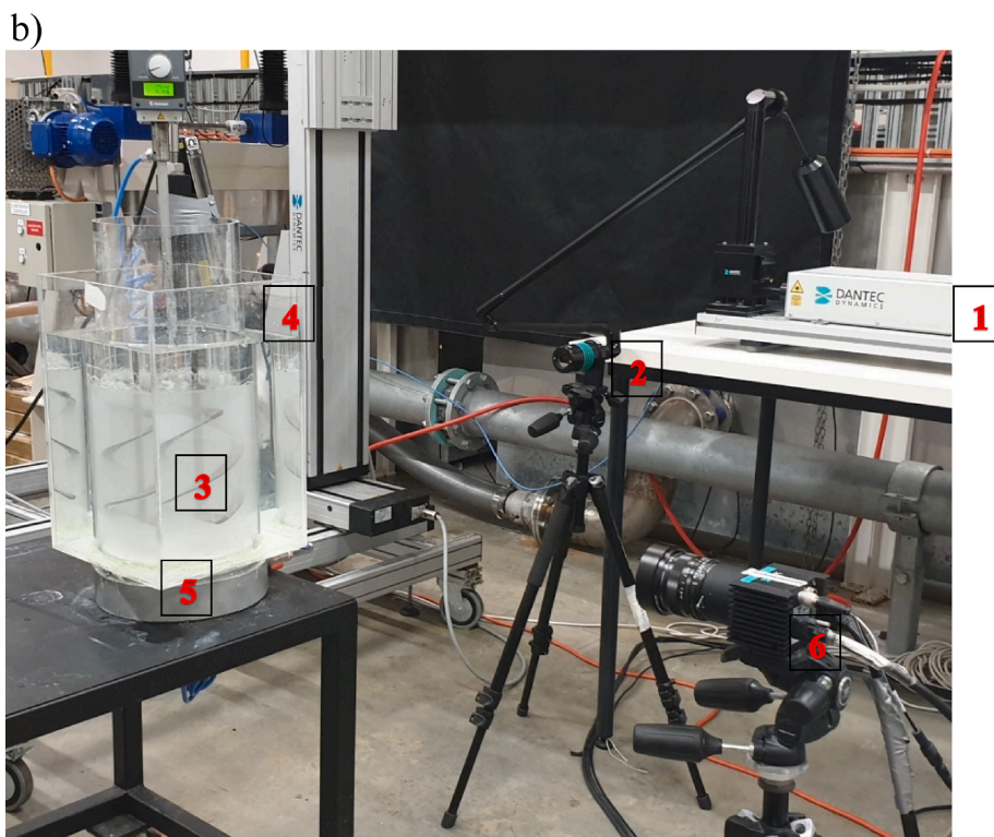
Fig. 2. (a) Schematic view of PIV system, and two-phase reactor; and (b) Experimental setup for PIV measurements.
