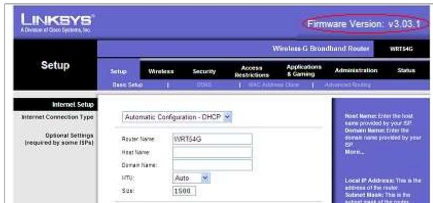
Figure 1: Firmware version specification on the Web Interface.
