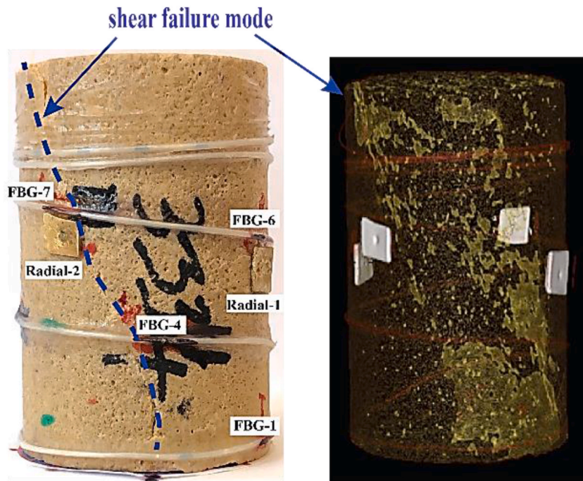
Fig. 7. Post-test photo (left) and 3D rendering of the main open structures and segmentation of X-ray CT images of the Sav-3334.
