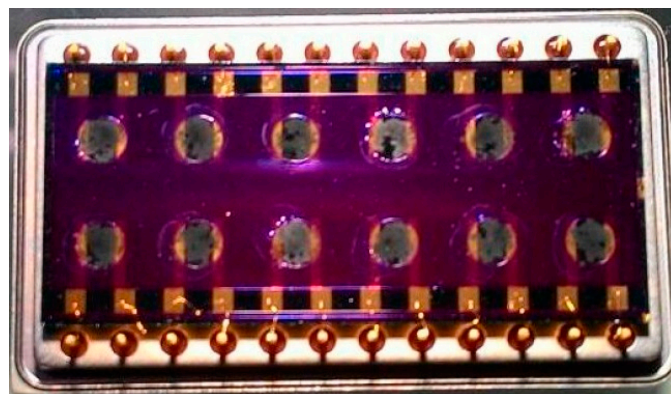
Figure 3. MWNT sensor array chip proposed by Wang et al. (Adapted from [92]).
