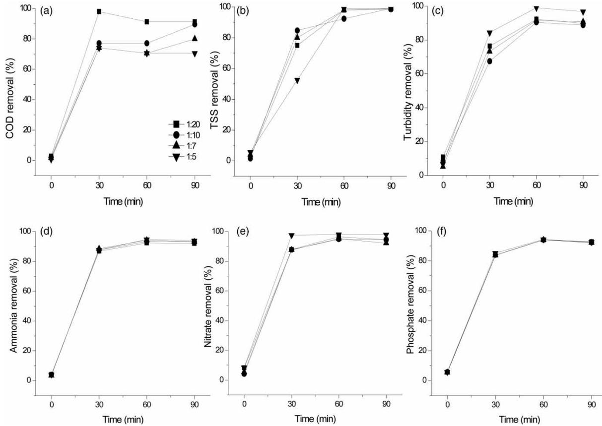
**Figure 3** | Variations in (a) COD, (b) TSS, (c) turbidity, (d) ammonia, (e) nitrate, and (f) phosphate removal efficiency by EC at 1:20, 1:10, 1:7 and 1:5 ratio of landfill leachate and municipal wastewater.
