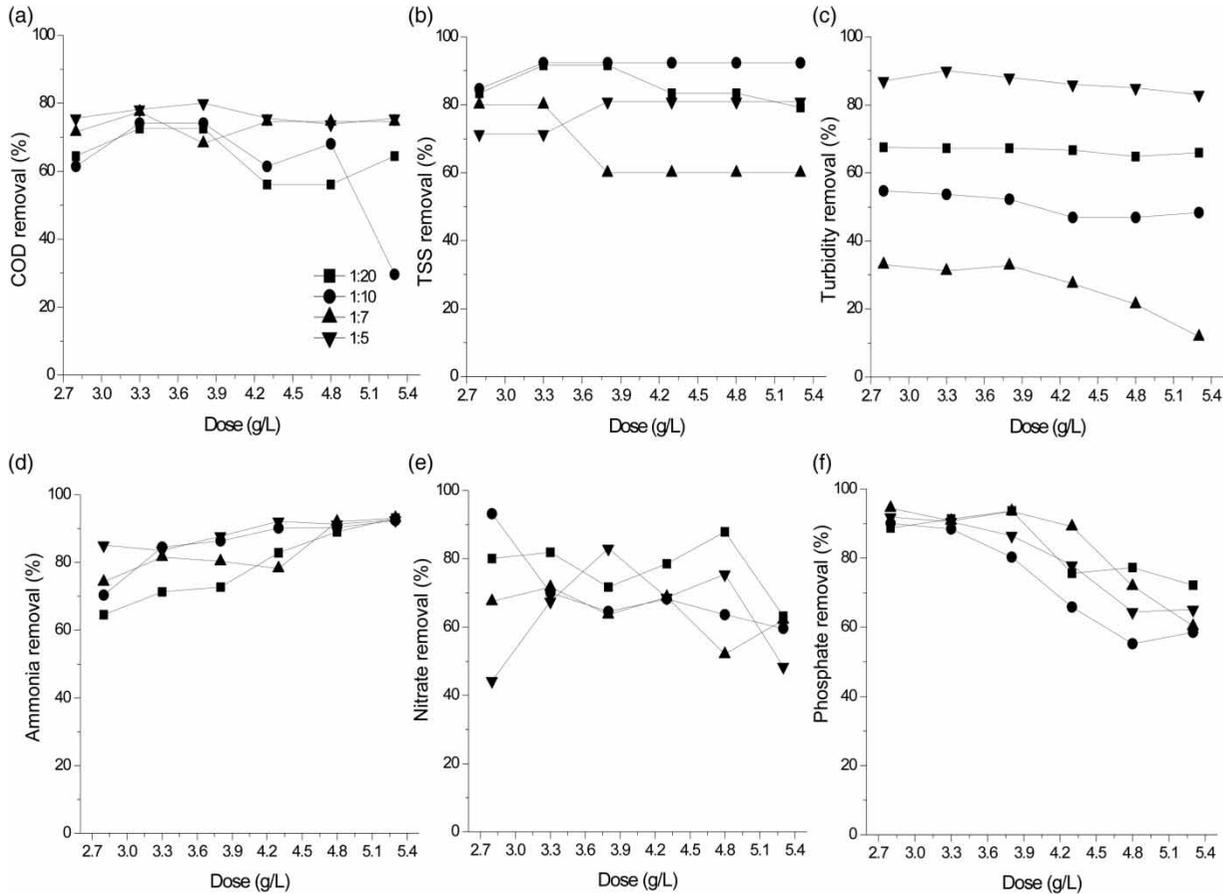
**Figure 1** | Effect of coagulant dosage during coagulation on the removal efficiency of (a) COD, (b) TSS, (c) turbidity, (d) ammonia, (e) nitrate, and (f) phosphate from landfill leachate and municipal wastewater at 1:20, 1:10, 1:7 and 1:5 ratio.
