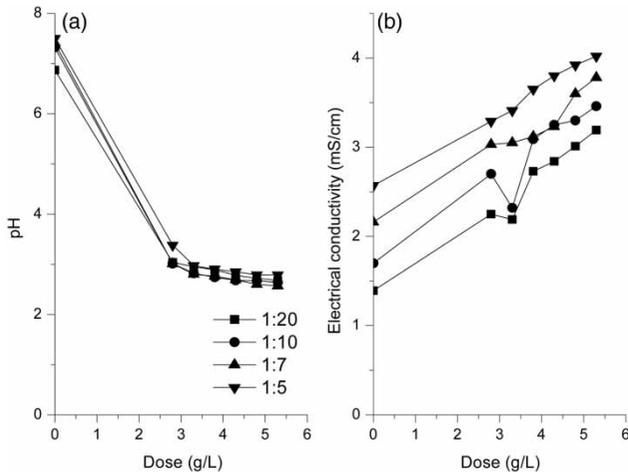
**Figure 2** | Variations in (a) pH and (b) electrical conductivity during coagulation at different doses of aluminum sulphate at 1:20, 1:10, 1:7 and 1:5 ratios of landfill leachate and municipal wastewater.
