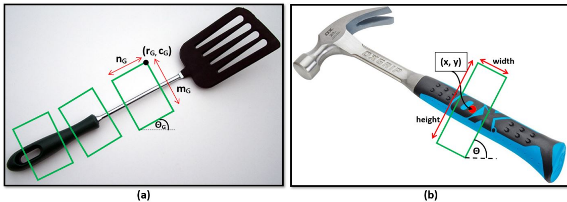
Figure 2. Grasping rectangle representations. (a) The representation by Jiang et al. [30]: Top vertex (r_G, c_G) , length m_G , width n_G and its angle from the x -axis, \theta_G for a kitchen utensil. There can be multiple ground truth grasps defined as shown. (b) The simplified representation by Redmon et al. [19] for a hammer, showing its grasp centre at (x, y) oriented by an angle of \theta from its horizontal axis. The rectangle has a width and height of w and h respectively.
