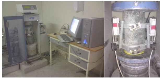
Figure 3. Compressive strength stress-strain tests apparatus.
