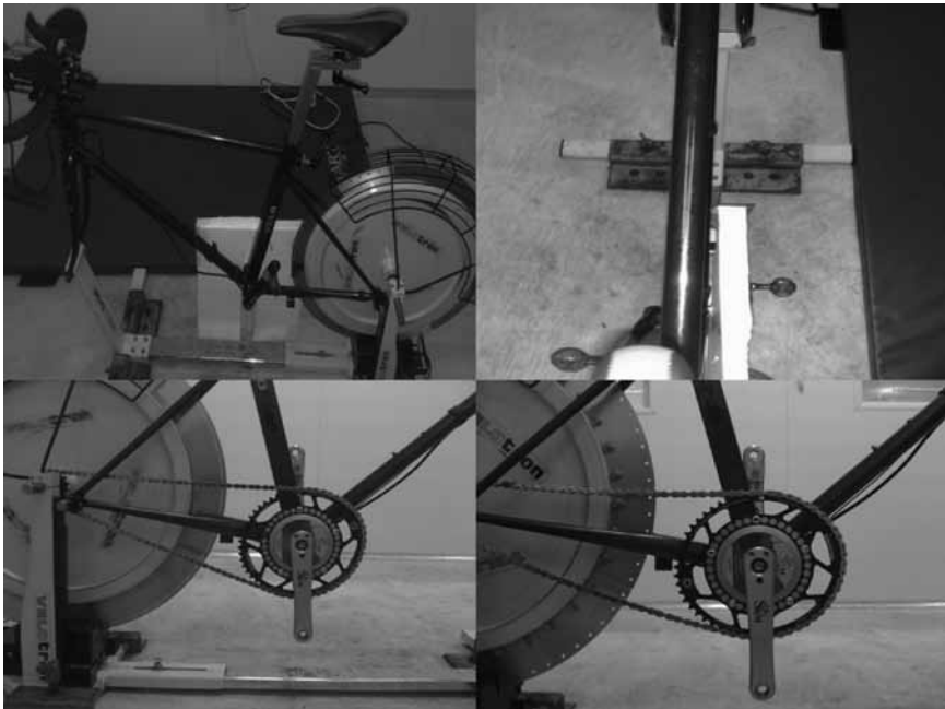
Figure 1 — Guard used to limit participant visibility of chainring (top-right and top-left) and orientation of the elliptical chainring in the elliptical 1 (bottom-left) and elliptical 2 (bottom-right) settings.
