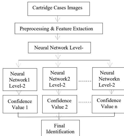
Fig.7. The proposed identification system
