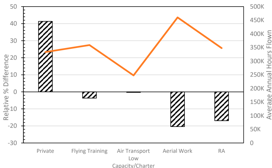
Figure 6. Delta values for type of flight operation. Expected (secondary axis), BITRE average annual hours for each type of operation (line plot).
