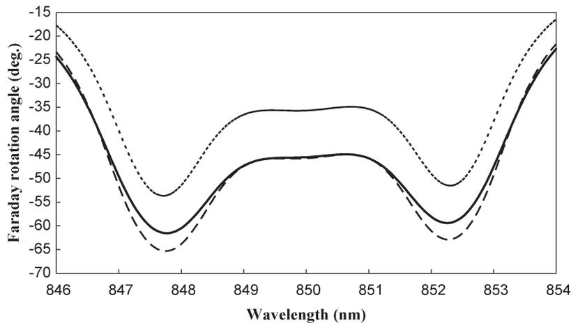
Fig. 2. Faraday rotation spectra of the optimized photonic crystal structure  $(NM)^3(MN)^7(NM)^7(MN)^2(NM)^2(MN)^7(NM)^5(MN)^1$  for various values of the absorption coefficient and gyration:  $A = 200 \text{ cm}^{-1}$ ,  $g = 0.02$  (dotted line);  $A = 200 \text{ cm}^{-1}$ ,  $g = 0.0256$  (dashed line);  $A = 300 \text{ cm}^{-1}$ ,  $g = 0.0256$  (solid line).
