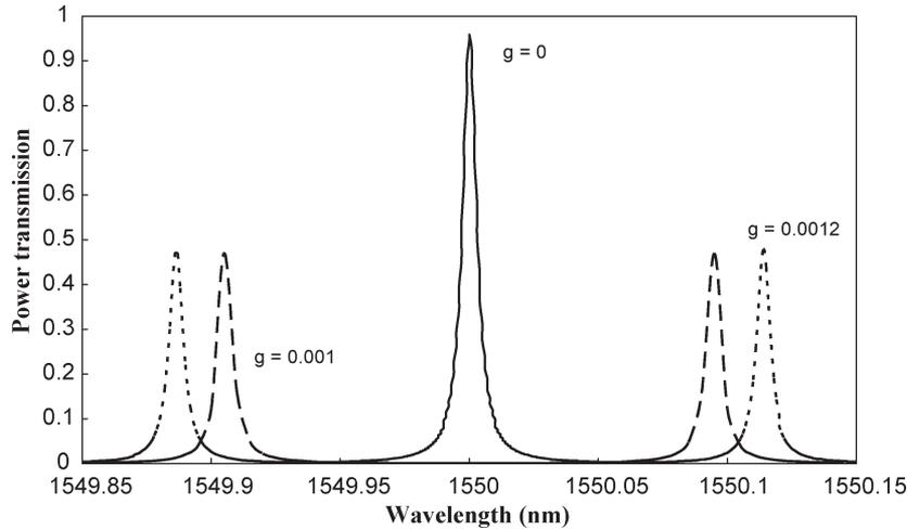
Fig. 4. Spectral transmission responses of the optimized MPC structure  $(NM)^{15}(MN)^1(NM)^1(MN)^{15}$  for  $\text{SiO}_2/\text{air}$  external media combination at various levels of induced gyration: Transmission in the absence of magnetic field (solid line), at  $g = 0.001$  (dashed line), and at  $g = 0.0012$  (dotted line).
