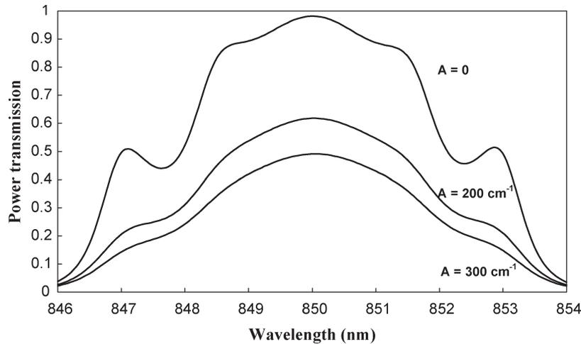
Fig. 1. Transmission spectra of the MPC structure  $(NM)^3(MN)^7(NM)^7(MN)^2(NM)^2(MN)^7(NM)^5(MN)^1$  optimized for broad-bandwidth low-rotation-ripple operation at 850 nm in the presence of saturated magnetization ( $g = 0.0256$ ). The effect of material absorption inside the magnetic layers is shown.
